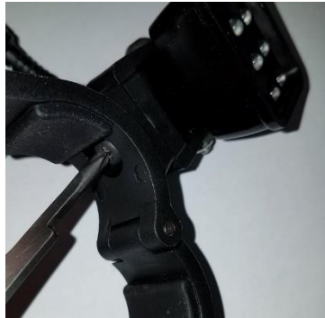
Figure 3 Loosening light retention bolt
