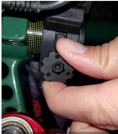
Figure 6 Retention bracket clamped on left handlebar end next to stem
