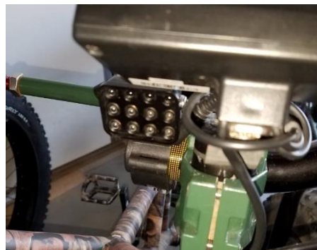
Figure 7 Light positioned under CycleAnalyst
