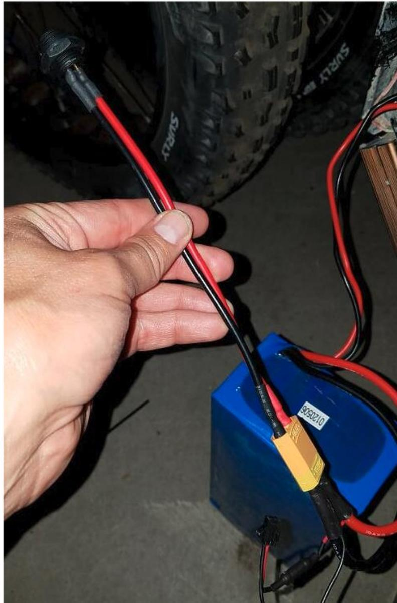
7. Plug the black connector on the battery reset cable into your battery charger. Make sure the charger has been disconnected from AC power (wall outlet) for at least 2 minutes before doing this step, otherwise you'll need to repeat this step.
