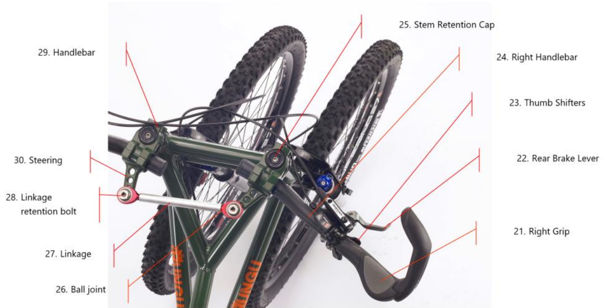
Figure 2 - Handlebar top view Kilimanjaro pre-2017
