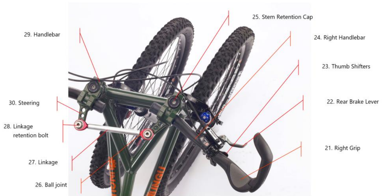
Figure 2 - Handlebar top view Kilimanjaro pre-2017
