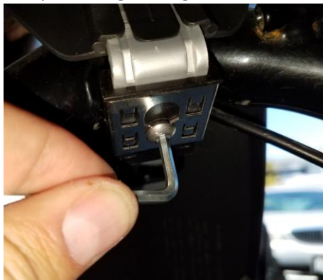
Figure 18 Tightening mounting block bolt to fasten fender to steerer tube
