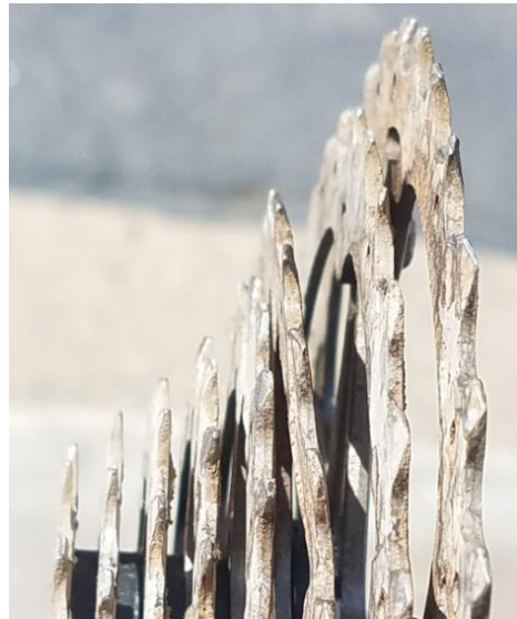
Bent 3rd gear cog resulting from gear change while hill-climbing and power level set to 5
