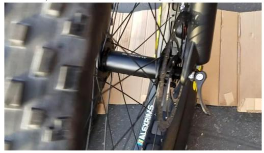
28. Tighten the end cap nut on the LEFT wheel and close the quick-release lever. As a guideline the end cap nut should begin to clamp onto the fork drop out when the lever points away from the wheel at a right angle.
