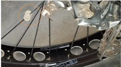
4. If you are replacing a magnet, place the magnet so that the face of the magnet faces the sensor and algins with the oblong recess on the sensor – it has the word "Bafang" embossed.
