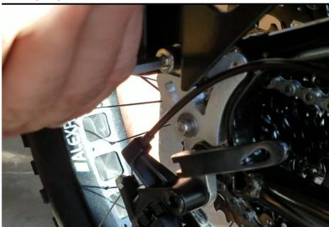
7. Use a 6 mm hex wrench to tighten all three screws, start with the screw on the mounting plate in the front.
