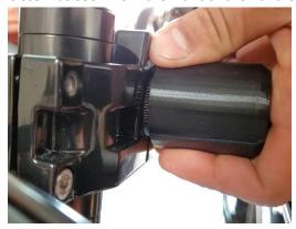
9. Replace the four bolts in the handlebar clamp and finger tighten.
