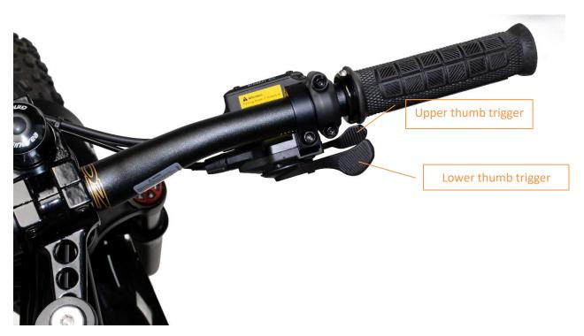
Each press of the thumb against one of the triggers indexes the gear. A long press of the Lower Thumb Trigger decreases the gear by one gear at a time starting in ninth gear. A short press of the Upper Thumb Trigger increases the gear by one gear at a time starting with first gear.
