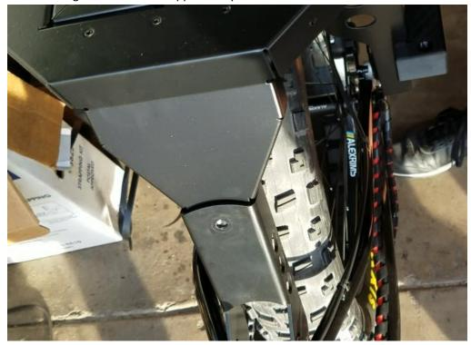
4. Align the front rack tab with the mounting bracket and place an M8 screw and washer through the mounting bracket hole. Thread the screw into the threaded hole on the front of the rack. Finger tighten.
