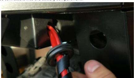
10. Working from the inside and the outside of the rack squeeze the grommet on the harness into place so that it covers the entire hole in the battery case and secures the cable harness.
