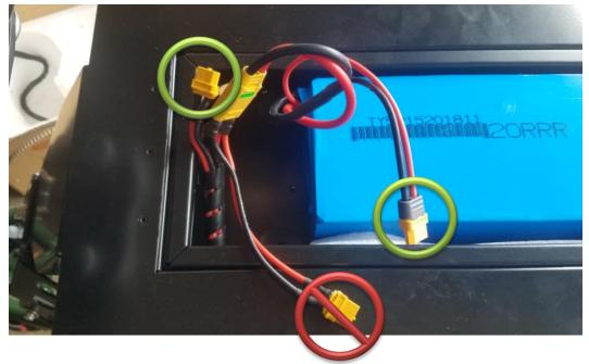
5. Plug both charger plugs to the connectors shown above.
