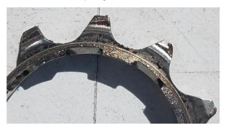
Same cog after three miles of acceleration from a full stop in 10<sup>th</sup> gear using power level 5. Note tooth damage. Also prior Shimano version of Cassette.
