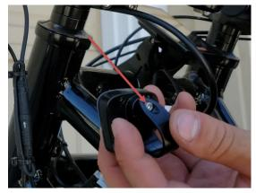
14. Mount the keypad onto the left handlebar and slide the keypad near the throttle.
