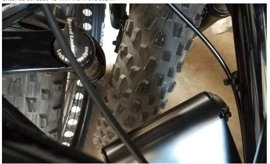
8. <u>Make sure the battery case covers are on and locked in place</u>. Verify that each battery case cover is in place and locked. If not, STOP. Lock each battery cover making sure to avoid pinching or severing wires.
