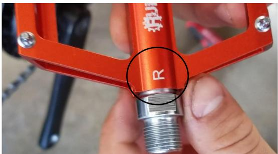
31. Use your fingers to thread the pedal shaft by inserting the threaded shaft into the crank arm. Then hold the threaded section of the pedal in the crank arm mounting hole and spin the entire crank arm in a counterclockwise motion as depicted below.
