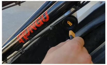
NOTE: You may hear a "pop" sound when you plug in the charger that comes from a spark that occurs inside the connectors when the two connectors mate. This is normal and a result of the potential difference between the battery and the charger.
