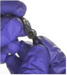
5. Pull the chain together and align the pins with the slots on the master link plates.
