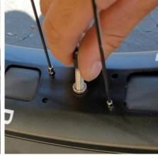
2. Unscrew the captive nut on the top of the presta valve to allow air to flow into the tire.
