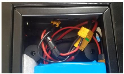
GOOD - cables placed away from door and key latch
