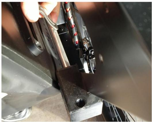
2. Adjust the upper quick-release catches using the adjustment knobs so that the catches fit between the two upper mounting blocks.
