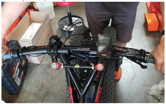
3. <u>Make sure each wheel is fully inserted into its dropout</u>. Look carefully at both sides of the quick release on each wheel and make sure that the quick release skewer ends are seated inside the recesses on the bottom of the forks for each fork and inside the slot in the frame of the rear
