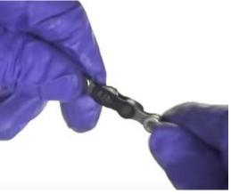
6. Rotate the chain so that the master link is above the chainstay and on the chain ring. With the rear brake engaged, you can step or use your hand on the right-side pedal to pull on the chain and set the master link. You should feel the master links "click" into place. Rotate the chain to verify the master links are set.
