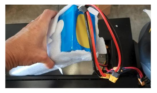
12. The small yellow connectors on each battery mate with the charger plugs on each charger. The connector is keyed, so there is only one way that the plug will fit.
