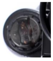
To stiffen or loosen the suspension, turn the right-side knob clockwise or counterclockwise respectively. All Dualies ship with the suspension at the loosest setting. If you find that the front-end dives too much, or that you are having difficulty turning on soft ground (sand, snow), increase the stiffness of both forks by turning the knob clockwise.
