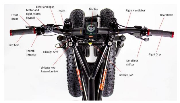
Figure 2 Steering assembly
