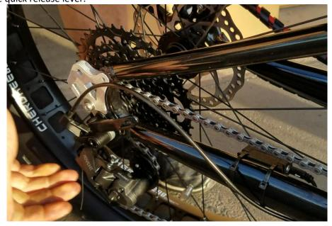
5. If the wheel doesn't appear to be vertical as in the picture below, loosen the quick release, realign and re-tighten the quick release.
