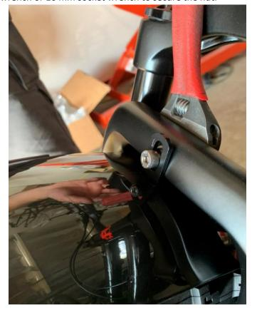
6. Use a 5mm hex wrench to continue threading the nut onto the screw
