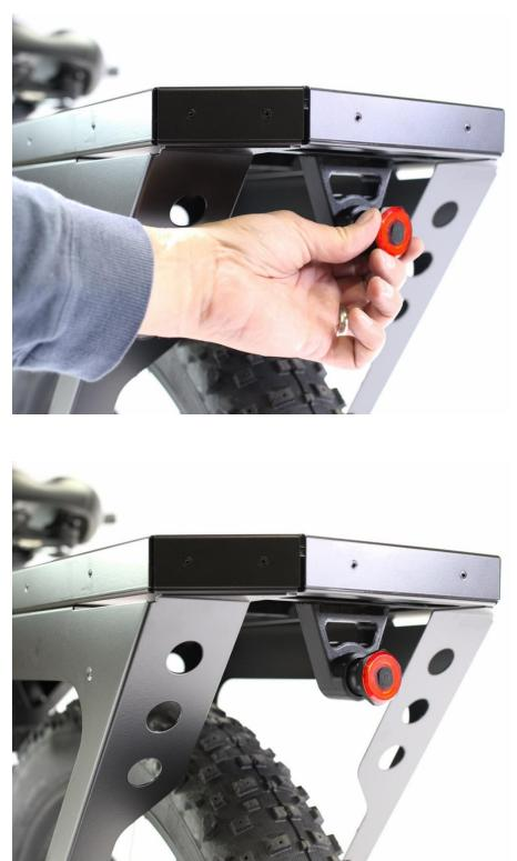
Screw the taillight into the mount socket.
