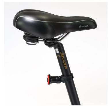
Screw the taillight into the socket.
