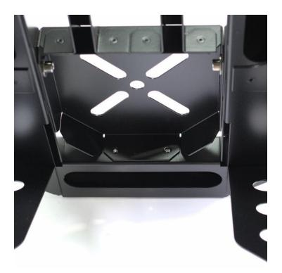
Align the mount with the screw holes as shown and use the 5mm hex wrench to install the first M6 screw and washer from the installation kit. Note that the socket side of the mount faces the rear of the cargo rack.
