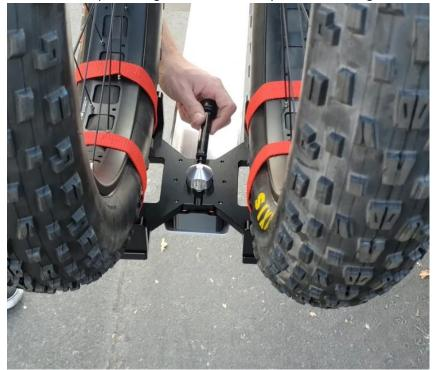
8. Replace the barrel lock and secure the lock pin with the key lock.
