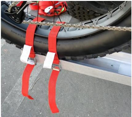
10. Use the soft-loop strap to tie down the front of the Rungu Dualie to the rack. Wrap a soft loop around the right head tube and hook the strap to the soft loop.
