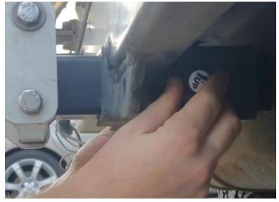
4. On the other side of the receiver place the spacer over the end of the pin, and then replace the barrel lock and remove the key to lock the pin in place.
