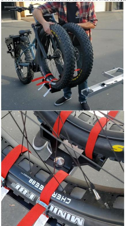
6. Lift the rear of the Rungu Dualie and pivot the bike around the wheel stand post and place the rear tire in the center of the hitch rack channel.
