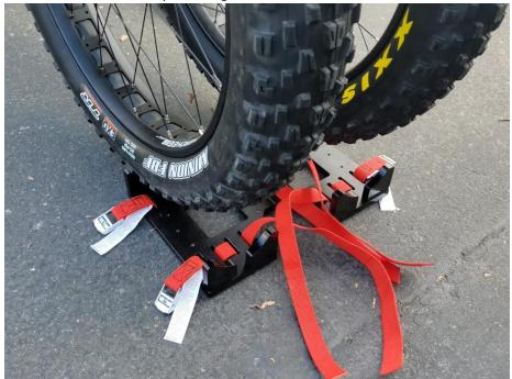
4. Secure each front tire with two tire straps. Tighten each strap
