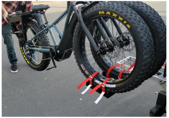
7. You can now roll the bike off of the rack, or lift the front wheels onto the ground. Orient the bike so the wheel stand is resting on the ground.
