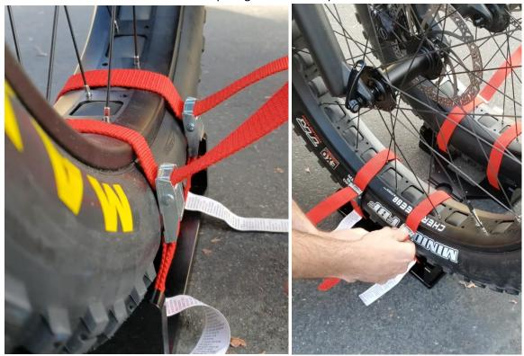
NOTE: Make sure the straps lay flat against the rim of the wheel and avoid twisting the straps before inserting them into the cam-buckles.
