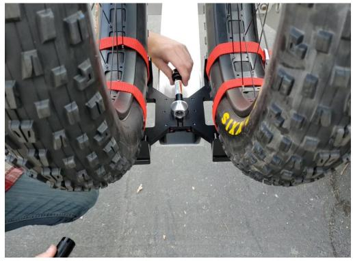
6. Lift the rear end of the Rungu Dualie, rotate the bike to be perpendicular to the rack and place the rear wheel on the ground.
