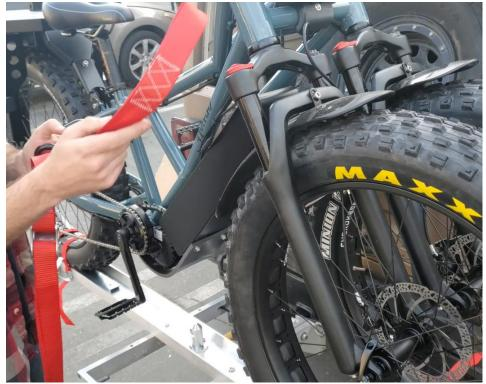
3. Remove both rear wheel tie down straps.
