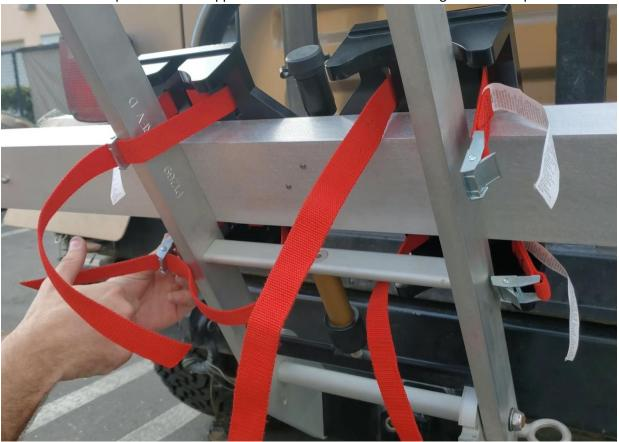
NOTE: Tightening the straps against the support bar prevents the wheel stand from rattling against the carrier rack.
