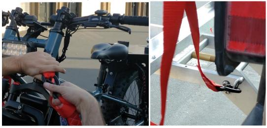
14. Hook the cam-buckle strap ends to the right-side seat stay tube below the cargo rack mount so that you pull down on the free end to tighten the strap.
