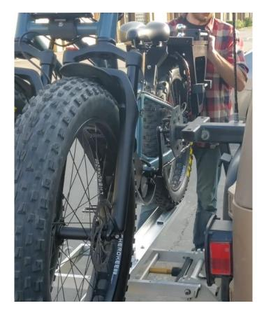
7. Insert the Lock pin through the wheel stand post to lock Rungu Dualie in position.
