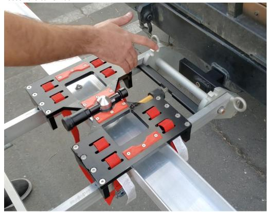
5. Pull on the position brace to pivot the rack vertically.
