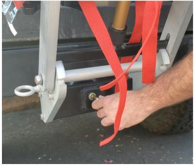
6. Check that Rungu Hitch Rack is secure by trying to rock it side to side.
