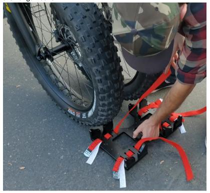
NOTE: Make sure you can access both ends of each wheel strap on the wheel stand – there are four straps in total
