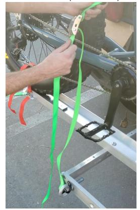
16. On the left side, hook the cam-buckle strap under the brake line behind the second tie down location.
