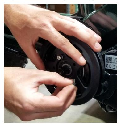
Finger-tighten the second screw, then install and finger tighten the remaining three screws and washers.
