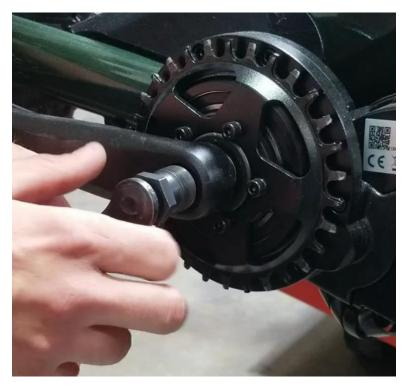
CAUTION: BE CAREFUL TO NOT CROSS THREAD THE CRANK PULLER MOUNTING NUT INTO THE CRANK ARM. FAILURE TO DO SO MAY DAMAGE THE CRANK ARM. CROSS THREADING IS NOT COVERED BY MANUFACTURER'S WARRANTY.
