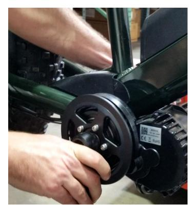
Insert the crank arm retention bolt and begin threading it into the drive axle.
