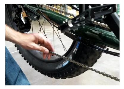
Use the master link pliers to spread the master links and snap the master link in place
