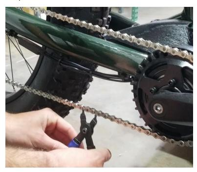
Drape the upper length of chain over the chainstay as shown below.
