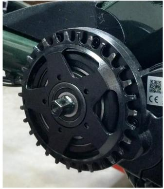
Place one of the M5x14 screws with a split washer through the chainguard and chainring.
