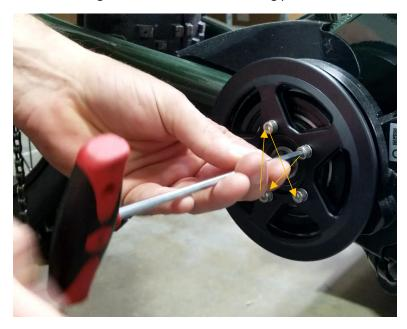
Finally use the chain whip to secure the chainring and fully tighten each screw using the same crossing pattern.
