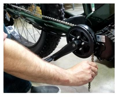
Use the master links to reconnect the return side (bottom) of the chain.
