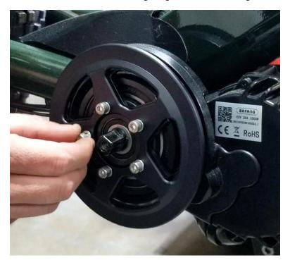
Use a 4 mm hex wrench to hand tighten each screw in a crossing pattern
