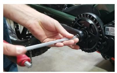
Install the crank puller into the crank arm.
