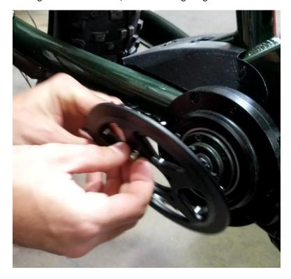
Install the next screw and split washer into a mounting hole on the opposite side of the spindle.
