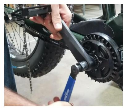
Unscrew and remove the crank arm puller from the crank arm.
