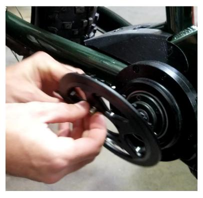
Align both with a mounting hole on the motor, install and finger tighten the screw.
