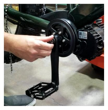
Use the 8 mm hex wrench to fully tighten the crank arm retention bolt to the drive axle.
