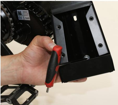
2. Align the skid plate mount so that the wide end is closest to the motor and use the 4 mm hex wrench to guide and fasten the screw into the lower threaded boss hand tight.
