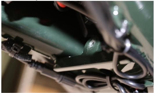
2. Align the hole in the rear of the skid plate with the threaded hole and use the 4mm hex wrench to loosely fasten the skid plate with the M5 x 18mm screw and washer.
