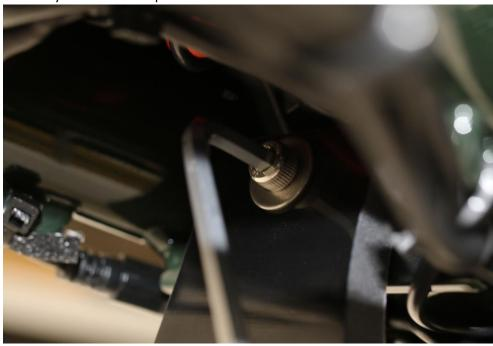
3. Align the front of the skid plate with one of the two threaded holes at the bottom of the skid plate mount. Insert an M6 x 18mm screw and washer and finger tighten (or use 6mm hex wrench).
