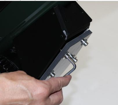
5. In a crossing fashion, progressively tighten each M6 screw against the skid plate until fully fastened against mount.
