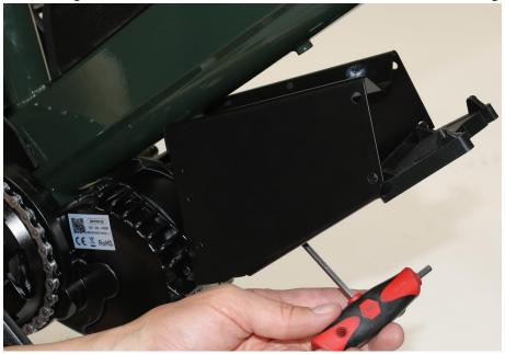
3. Use the second M5 x 14mm screw and washer to fasten the mount through the upper slot in the skid plate mount to the upper boss. Fully tighten.
