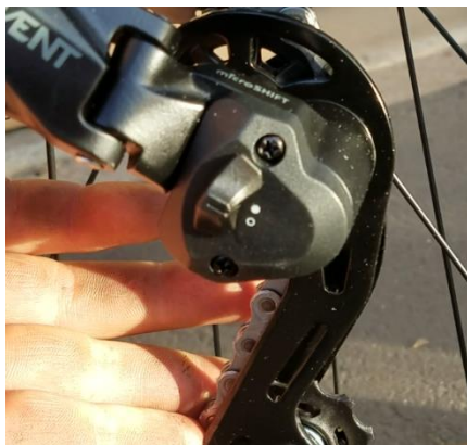
Figure 1 Clutch enabled - switch aligned with dot
