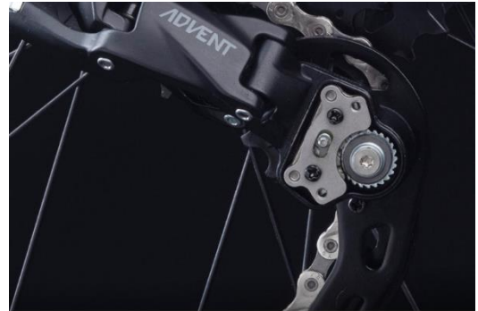
Figure 3 Cutaway view of Advent clutch mechanism
