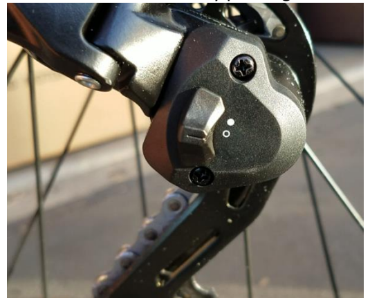
Figure 2 Clutch disabled - switch aligned with circle
