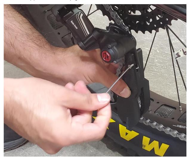
Finish installing all three fasteners and fully tighten each one by hand.
