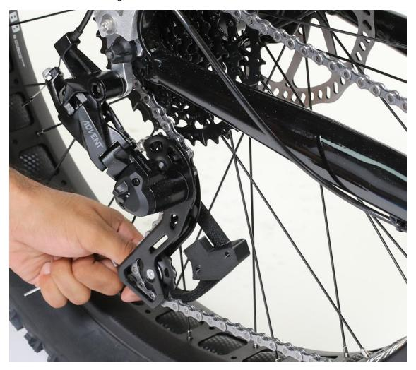
The inner guard plate will stay in place while you prepare the outer guard plate.
