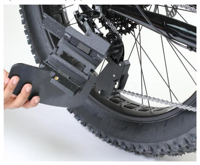
Place the clamshell in front of the derailleur and under the chain stay.
