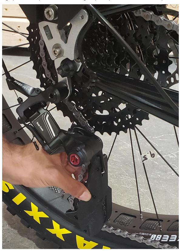
With both guard plates aligned with the derailleur cage, use the 2mm hex wrench to install the first M3 screw in the top position. Do not fully tighten.
