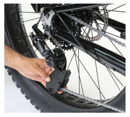
Use the 2mm hex wrench to install the first M3 screw in the middle position
