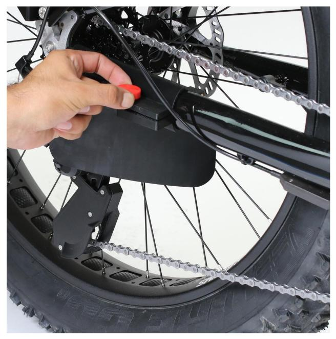
Finally, use your hand to try and rotate the cassette blocker around the chain stay. If the cassette blocker rotates without resistance, remove the cassette blocker and add one more layer of foam tape to the top or bottom on top of the existing tape. Re-install the cassette blocker and try again. If the cassette blocker still rotates without resistance add the second piece of foam tape.
