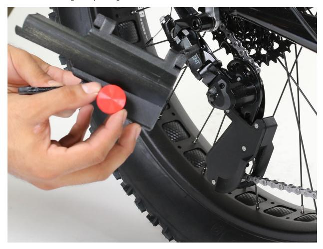
Remove the fastening bolt and open the cassette blocker "clam shell" as shown below.
