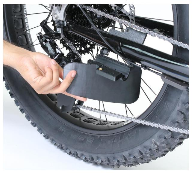
Slide the top section of the clamshell under the chain and derailleur cable. Then pinch the top and bottom sections together while orienting the back of the chain stay against the rear drop out. The tab at the back of the upper section should be on the outside of rear dropout
