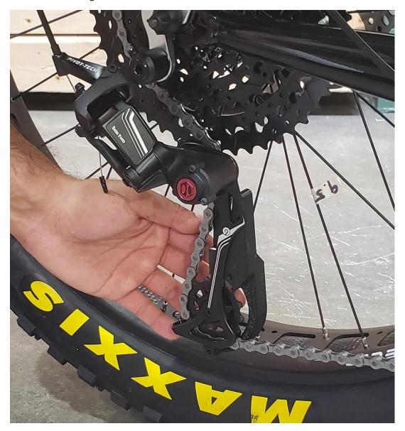
At the same time, align the outer guard plate with the inner guard plate and the derailleur cage. Apply slight pressure with your thumb to the outer guard plate – you should feel it "click" into place.
