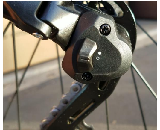
Figure 7 Clutch disabled - switch aligned with circle
