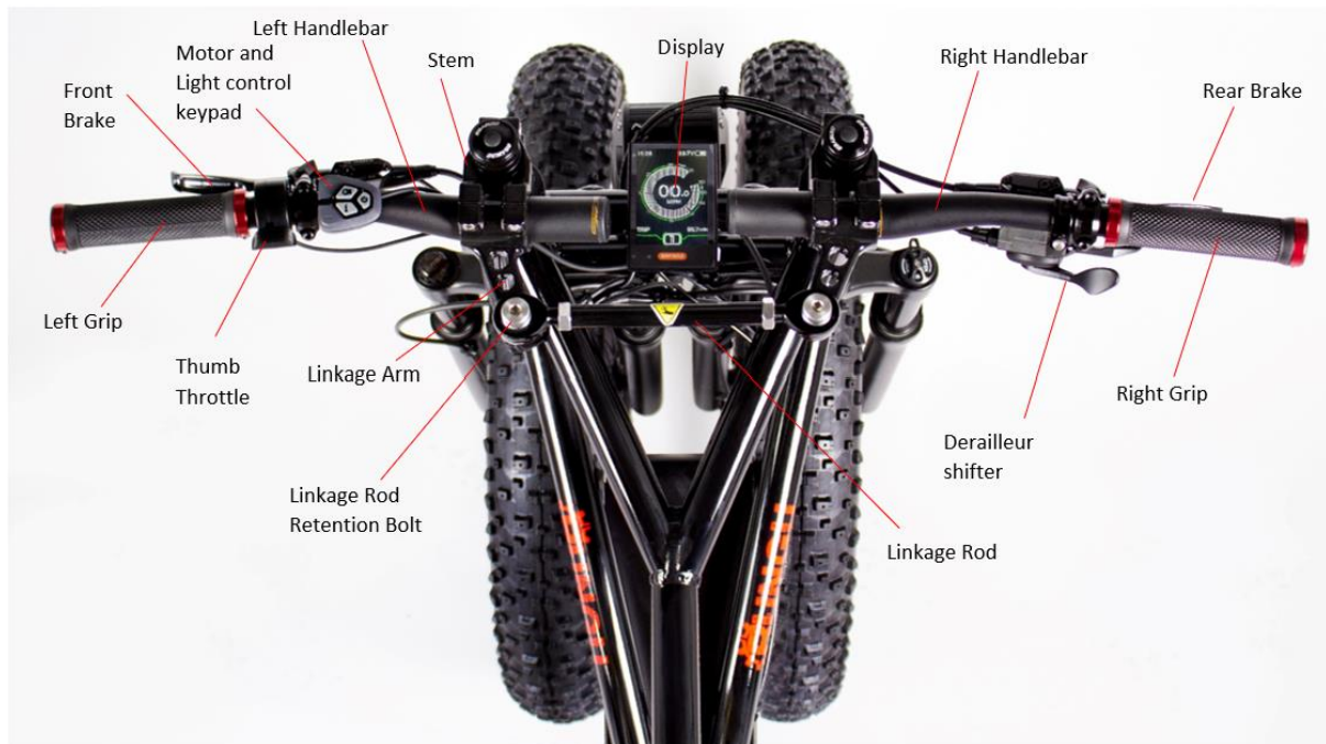
Figure 2 Steering assembly
