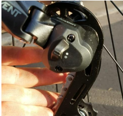
Figure 6 Clutch enabled - switch aligned with dot
