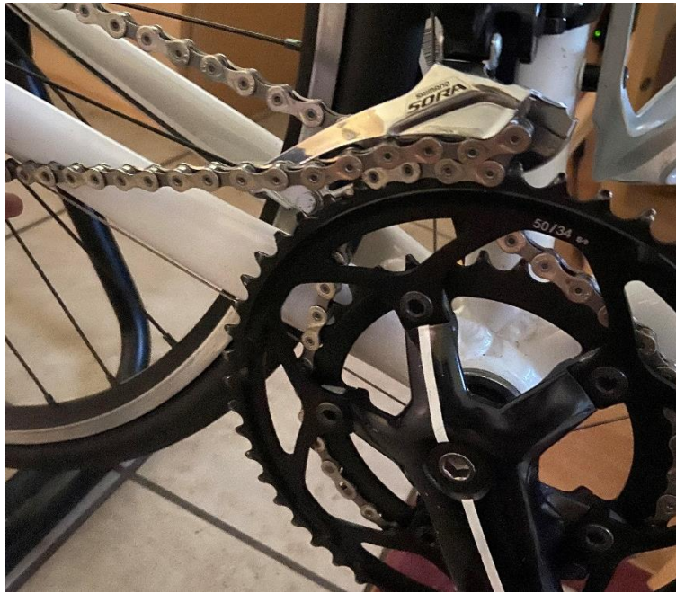
Figure 9 Image of chain suck - note chain wrapped around chainring
