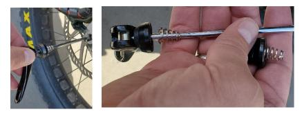
3. Insert the skewer with the M10 lock washer from one side of the bike so that the threaded end of the skewer is accessible on the other side.
