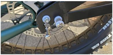
3. Make sure that the Front Fork Dropouts are free to mount on each side by releasing locking mechanism to open the Front Fork Dropouts.
