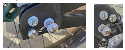
6. Press the lock release button and pivot the lock down so that it captures the spindle on each side.
