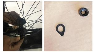
8. Install the rear wheel into the dropouts of the Wheel and Rack frame.
