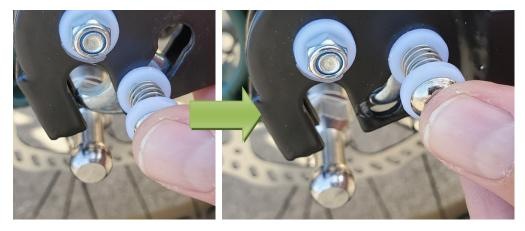
5. Position the fork dropouts over the spindles on either side of the rear wheel, raise the kickstand and lower the dropouts onto the Rungu Hitch.
