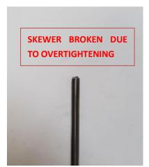
WARNING – DO NOT TIGHTEN THE SKEWER BEYOND ONE AND A HALF TURNS PAST FINGER TIGHT. DOING SO MAY CAUSE SKEWER TO SEPARATE AND FREE REAR WHEEL FROM FRAME, WHICH MAY CAUSE AN ACCIDENT LEADING TO RIDER INJURY OR DEATH.
