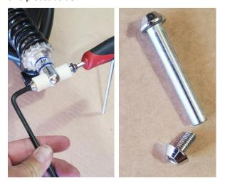
3. Install the Wheel and rack Frame into the bracket on the back of the Cargo Frame so that the pivot aligns as shown below – insert the pivot barrels into either side of the bracket to hold the Wheel and rack Frame in place with the Cargo frame.
