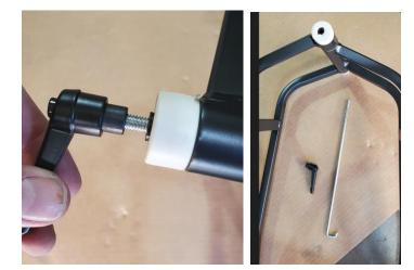
12. Unscrew the tightening lever from the mandrel on the Front Fork. Remove the mandrel and place aside.
