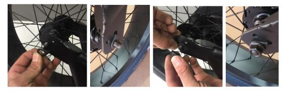
10. Use 15 mm socket wrenches, box wrenches or adjustable wrenches to tighten both nuts simultaneously.
