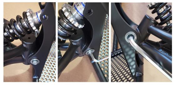
5. Align the upper pivot of the shock absorber with the holes in the bracket. Insert the sex bolt nut through the bracket and the upper pivot. Use the two 5 mm hex wrenches to tighten the sex bolt in place.
