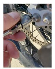
4. Before continuing make sure that the M10 lock washer is flush against the frame dropout and not caught in the dropout.
