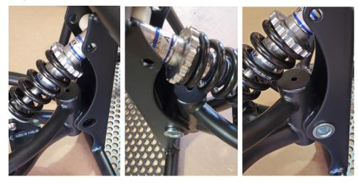
4. Insert the screw from step 1 into the shorter of the two barrels. Use the 6 mm Hex Wrench to engage the threads in the longer barrel. Use the 10 mm Hex Wrench in the longer barrel to secure the barrel. Tighten the screw with the 6 mm Hex Wrench.
