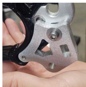
Cargo Rack Mount with 2xM5x18 bolts, 2xm5 washers, 1x M6x30TL bolt and 1x M6 washer.
