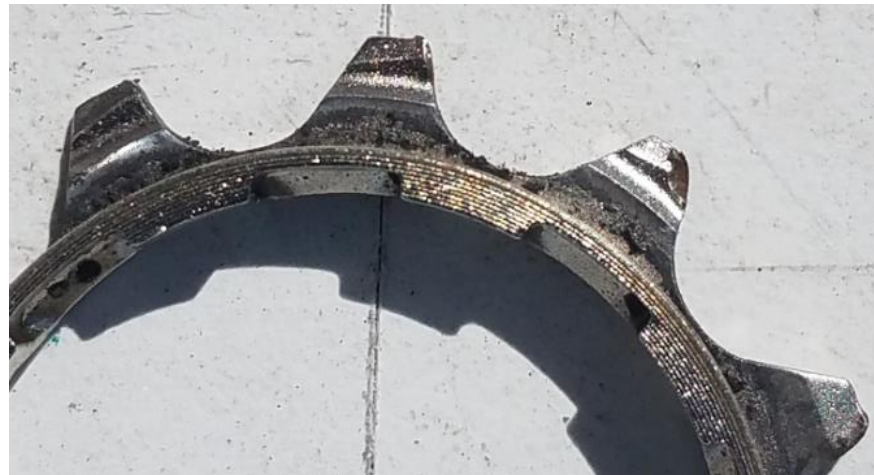
Same cog after three miles of acceleration from a full stop in 10 th gear using power level 5. Note tooth damage. Also prior Shimano version of Cassette.
