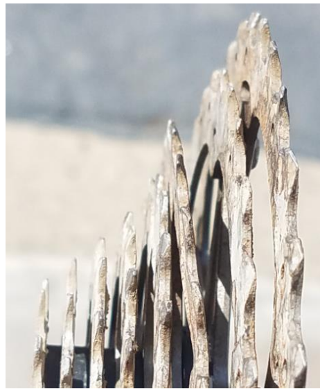
Bent 3rd gear cog resulting from gear change while hill-climbing and power level set to 5 – older Shimano cassette
