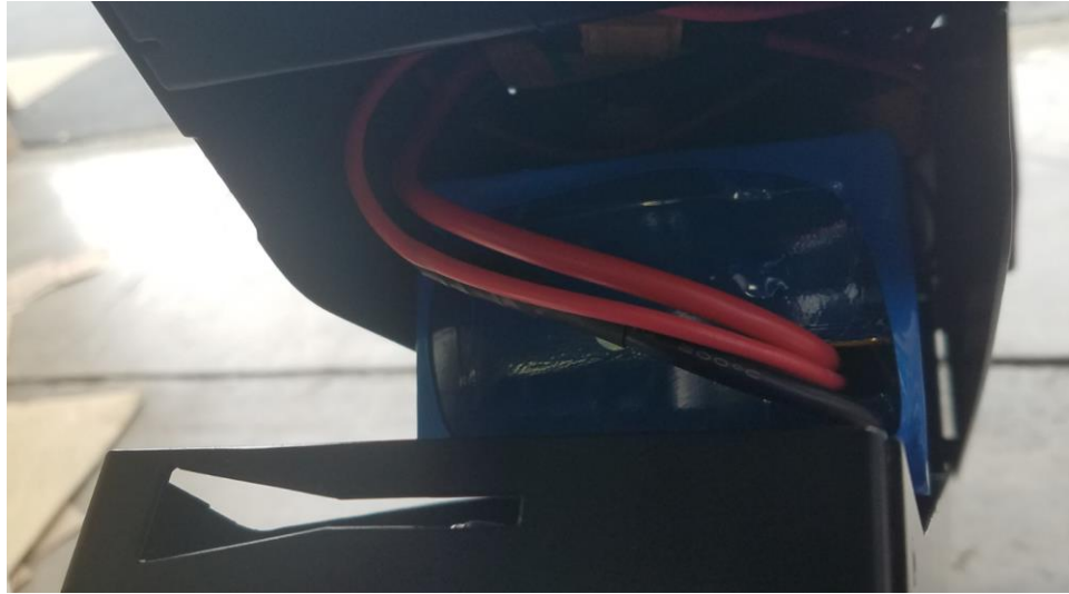
GOOD - cables positioned away from cover
