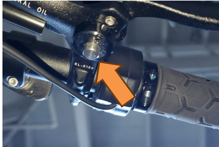
Figure 5 Parking brake button under left brake lever
