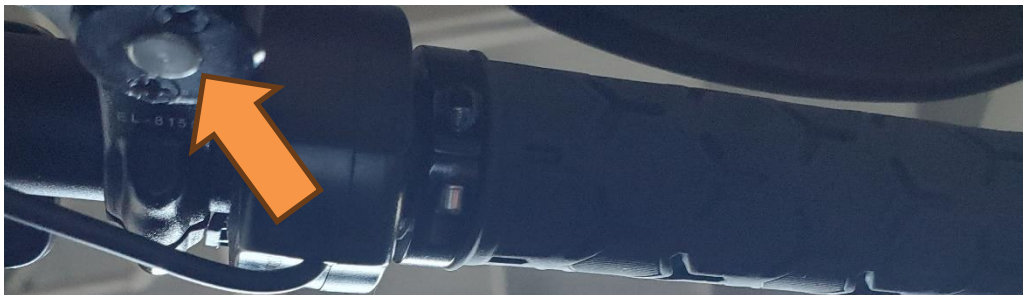
Figure 6 Button engaged, front parking brake on
