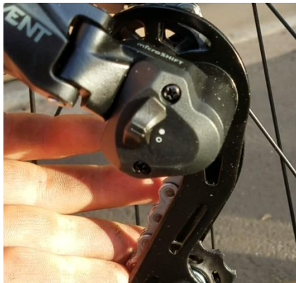
Figure 7 Clutch enabled - switch aligned with dot
