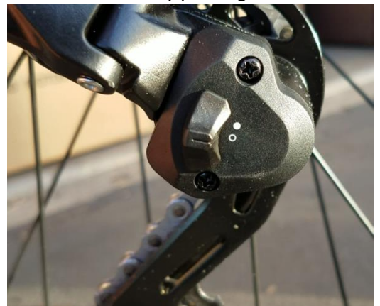
Figure 8 Clutch disabled - switch aligned with circle
