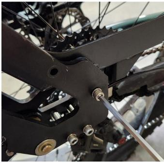
• Insert the M6 x 18 black oxide screw where shown and finger tighten.
