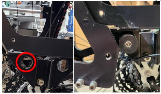
Hold the centering spacer and M6 standoff in place while rotating the right half of the kickstand.
