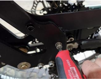
• Fully tighten the M6 x 18 black oxide screw using a 5mm hex wrench.
