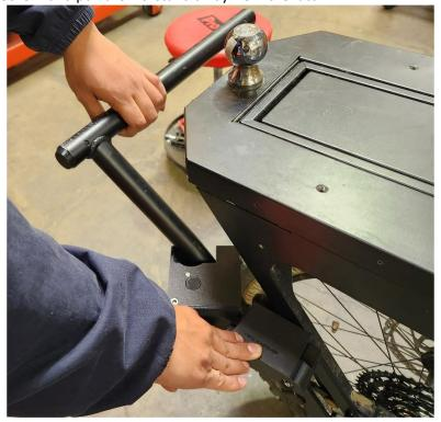
• Pull the kickstand foot down to the ground and step on it to keep it in place as shown.
