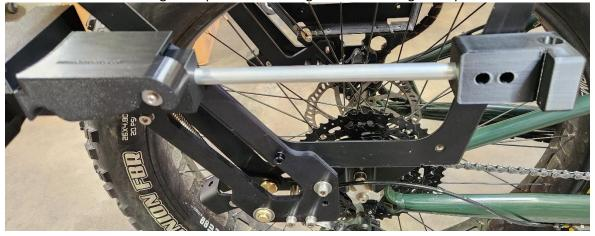
• Rotate the cargo rack pannier mount. You may need to rotate the mount to fully embed the bar into the recess of the mount.
