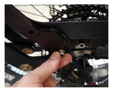
• Fasten the M6 x 50 screw using a 5mm hex wrench. Do not fully tighten, this will be done in a later step.
