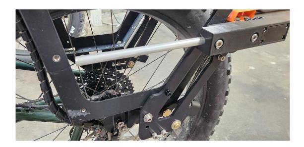
Insert the lower cargo rack pannier mounting bar into the cargo rack pannier mount as shown.
