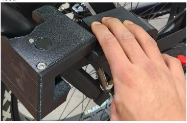
• Orient the kickstand foot as shown and remove the kickstand wedge from the left side.
