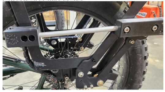
• Fasten the M8 x 35 screw using a 6mm hex wrench. Fully tighten the screw.
