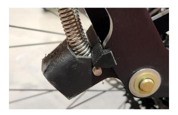
• Inert the M6 x 22 screw with an M6 washer into the foot mounting bracket as shown below. Use a 5mm hex wrench to keep the screw in place. If you have not put a drop of thread locker on the screw threads; do so now.
