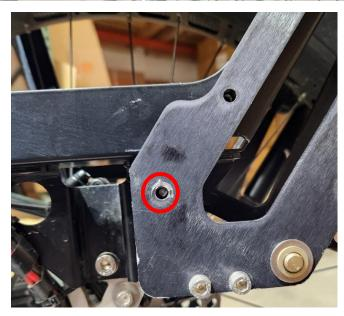
• Insert the M6 x 50 screw where shown and finger tighten. Be sure to include an M6 split washer as shown.
