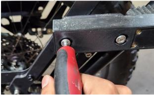
• Fully tighten the M6 x 50 screw using a 5mm hex wrench.
