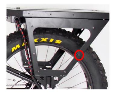
• Use the M8 x 35 screw with a 6mm hex wrench to fasten the left half to the left side of the stand. Be sure to include an M8 washer. Do not fully tighten, this will be done in a later step.
