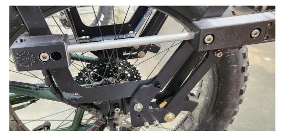
• Insert the lower cargo rack pannier mounting bar into the right half of the kickstand as shown.
