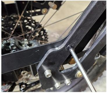
• Fully tighten the M8 x 35 screw using a 6mm hex wrench.
