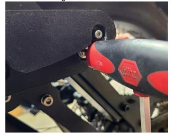
• Fully tighten the M6 x 50 screw using a 5mm hex wrench.
