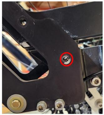
• Insert the M6 x 50 screw where shown and finger tighten. Be sure to include the M6 split washer as shown below.
