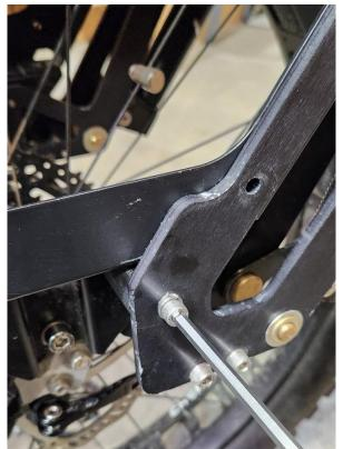
• Insert the M6 x 18 black oxide screw where shown and finger tighten.
