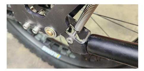
• Fully fasten the kickstand foot to the assembly by tightening both M6 x 22 screws using a 5mm hex wrench.
