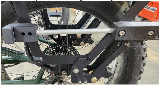
• Rotate the cargo rack pannier mount into position. You may need to rotate the mount to fully embed the bar into the recess of the mount.
