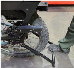
• Grab the back of the cargo rack and pull backwards to set the kickstand.
