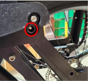
• Fasten the M8 x 35 screw using a 6mm hex wrench. Be sure to include an M8 washer. Do not fully tighten, this will be done in a later step.
