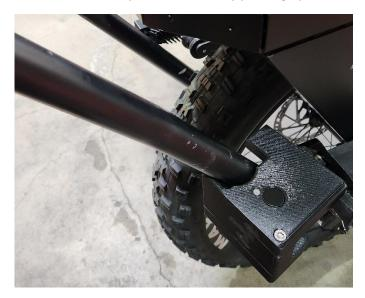
• Insert the M6 x 22 screw into the kickstand foot and fasten using a 5mm hex wrench. Once the screw has been fully tightened, back it off by half a turn. The screw will be fully tightened in a later step.
