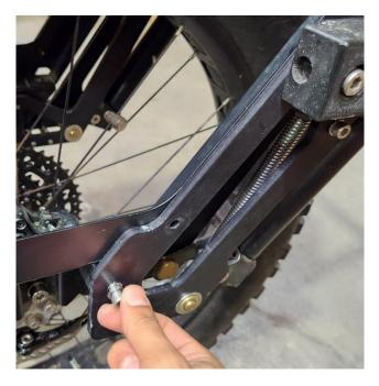
• Fasten the M6 x 50 screw using a 5mm hex wrench. Do not fully tighten, this will be done in a later step.
