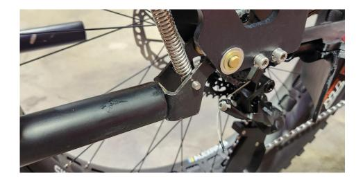
Re-orient the kickstand foot as shown and ensure that the kickstand latch is in the closed position.
