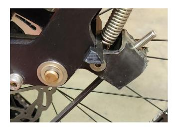
• The kickstand foot is currently oriented as shown in the first image. Rotate the kickstand foot to get it into the position shown in the second image.
