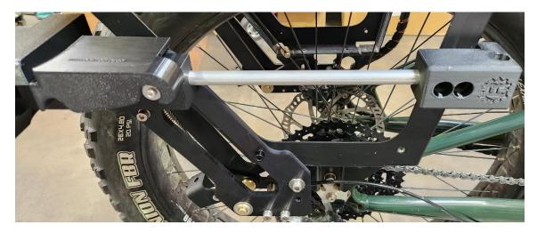
• Fasten the M8 x 35 screw using a 6mm hex wrench. Fully tighten the screw.
