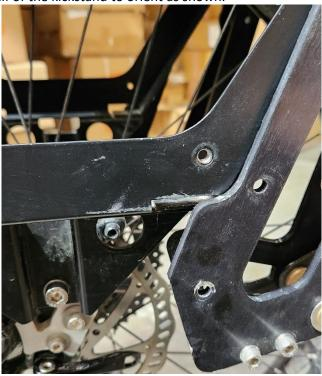
• Insert the M6 standoff into the centering spacer as shown.
