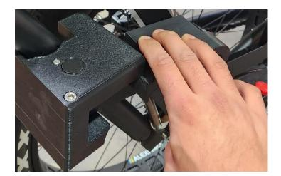
Rotate the right foot mounting bracket by hand as shown.
