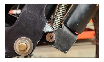
Press down on the "PRESS TO RELEASE" trigger as shown below to release the kickstand latch and kickstand foot.
