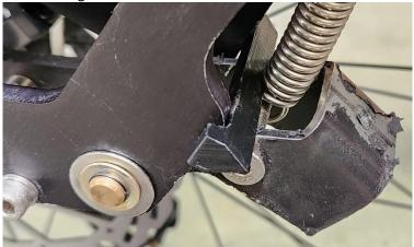
• Inert the M6 x 22 screw with a M6 washer into the foot mounting bracket as shown below. Use a 5mm hex wrench to keep the screw in place. . If you have not put a drop of thread locker on the screw threads; do so now.
