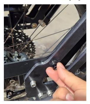
• Fasten the M6 x 18 black oxide screw using a 5mm hex wrench.
