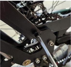
• Fully tighten the M8 x 35 screw using a 6mm hex wrench.
