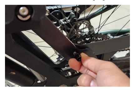
• Fasten the M6 x 18 black oxide screw using a 5mm hex wrench. Do not fully tighten, this will be done in a later step.
