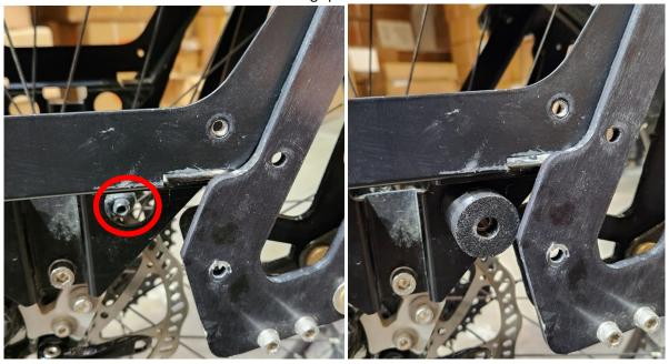
Hold the centering spacer and M6 standoff in place while rotating the left half of the kickstand.
