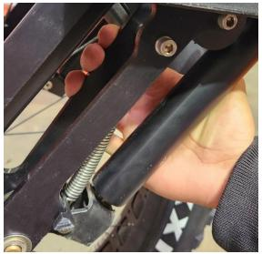
• Fasten the M6 x 22 screw into the kickstand foot using a 5mm hex wrench. Do not fully tighten, this will be done in a later step.
