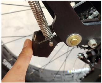
• Push down on the foot mounting bracket and Insert the kickstand wedge as shown.
