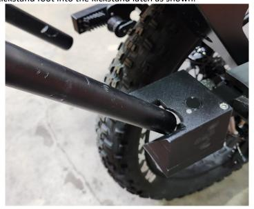
• Rotate the kickstand latch into the position shown by pushing upwards on the kickstand foot.
