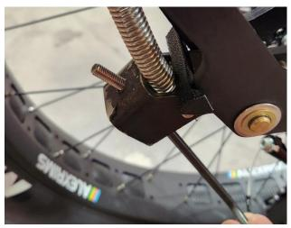
Position the kickstand foot into the kickstand latch as shown.
