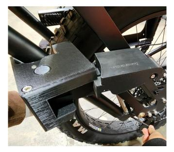
Rotate the partially fastened kickstand foot to orient it as shown and remove the kickstand wedge.
