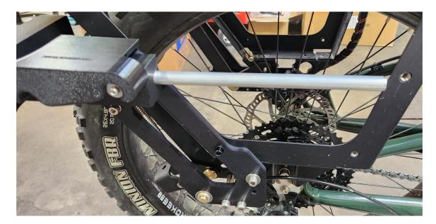
Insert the lower cargo rack pannier mounting bar into the cargo rack pannier mount
