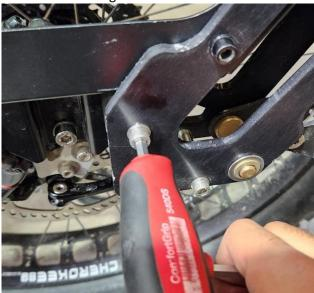
• Fully tighten the M6 x 18 black oxide screw using a 5mm hex wrench.
