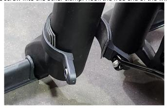
12. Fasten the M5 x 12 screw using a 4mm hex wrench. Do not fully tighten; this will be done in a later step.
