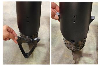
5. Insert a M5x25 SHCS Mud Diverter Screw with M5 washer into a top mounting bracket as shown below.
