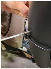
8. Use the 4 mm hex wrench to tighten both M5x25 SHCS Mud Diverter Screws hand tight to secure the stay and the Mud Diverter.
