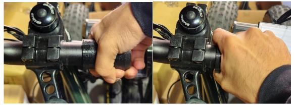
4. After you have replaced the end stop, the gap between the edge of the end stop and the side of the handlebar clamp should be the same or equivalent to the gap you noted for the prior endstop.
