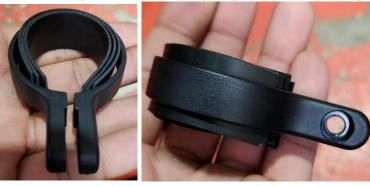
4. Insert a M5 nylock nut into each clamp as shown.
