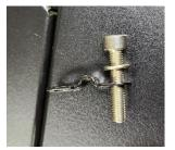
6. Install the M5x25 SHCS Mud Diverter Screw and assembly in the bottom hole of the Mudguard and engage the threads of the Mud Diverter so that the top mounting bracket is loose enough to align the stay bracket in the assembly as shown below.
