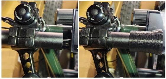
3. Finish installing the extended front fender handlebar end stop by pushing it while twisting back and forth.
