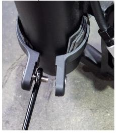
10. Fasten the M5 x 12 screw using a 4mm hex wrench. Do not fully tighten; this will be done in a later step.
