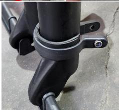
6. Lower the clamp and rubber spacers down until the rubber spacers meet the dropout circled below.
