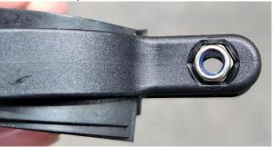
5. Spread the clamp apart and place it onto the right-side stanchion of the first fork as shown. NOTE: Orient the clamp so that the M5 nylock nut faces the wheel side of the fork as shown.
