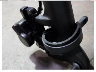
8. Lower the clamp and rubber spacers down until the rubber spacers meet the dropout circled below.
