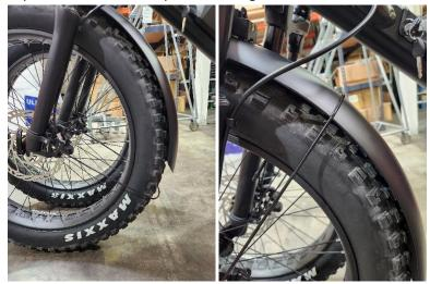
4. Slide a Mud Diverter under the Mudguard and align the holes in the Mud Diverter with the holes at the bottom of the Mudguard as shown below.
