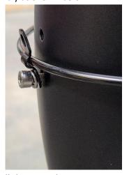
7. Use the 4mm Hex Wrench to install the second M5x25 SHCS Mud Diverter Screw to fully capture the stay.
