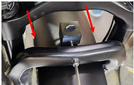
3. Rotate the stay to position it over the top of the Mudguard.
