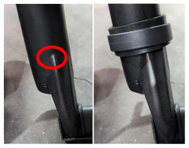
7. Place the next clamp on the left-side stanchion circled below. Spread the clamp apart and insert the side with M5 nylock nut between the brake mount and the stanchion.
