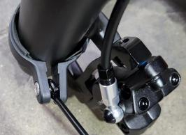
11. Insert a M5 x 12 screw into the other clamp. Hook the free end of the wire stay onto the screw.
