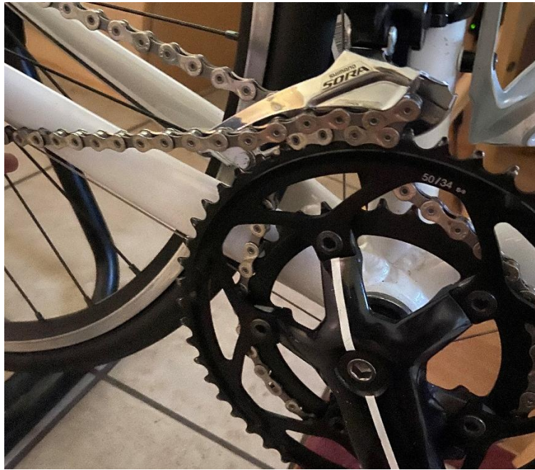
Figure 11 Image of chain suck - note chain wrapped around chainring
