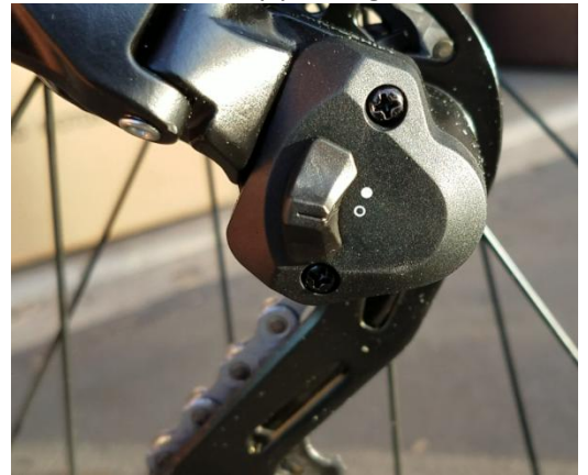
Figure 9 Clutch disabled - switch aligned with circle
