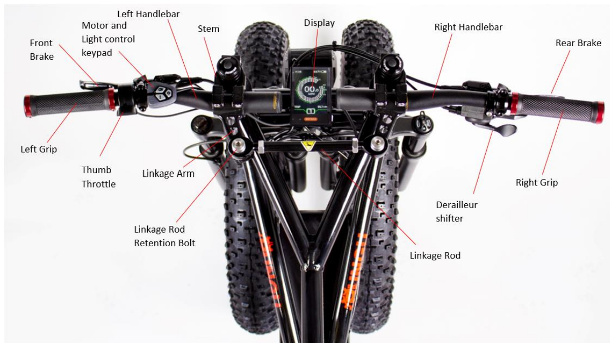
Figure 2 Steering assembly
