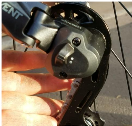
Figure 8 Clutch enabled - switch aligned with dot
