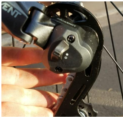
Figure 8 Clutch enabled - switch aligned with dot
