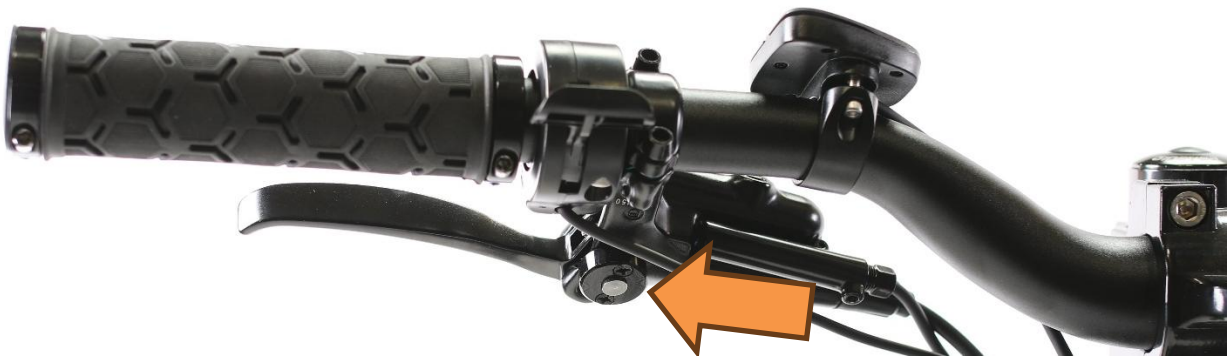
Figure 7 Button engaged, front parking brake on
