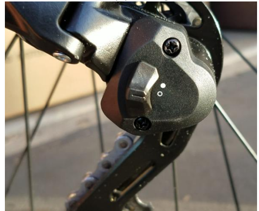
Figure 9 Clutch disabled - switch aligned with circle
